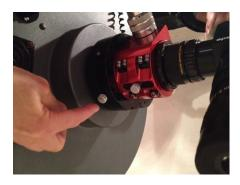
If you cannot get focus by turning the focussing knobs, the black mirror focuser knob may need turning to bring focus within the range of the focuser.
