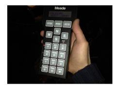
The number keys on the left hand side also have an effect – by pressing 7 the telescope will move quickly, less quickly on 4 and slower on 1. 0 slews at 2x sidereal rate accurate pointing.
